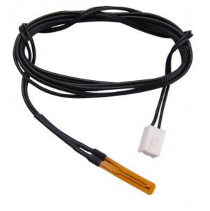
NOTE: This sensor will only work with Koolance products which use 50K Ohm @25°C sensors (introduced before 2011). Flat thermistor temperature sensor compatible with Koolance multi-sensor systems. Wire length = 30" (76cm).
