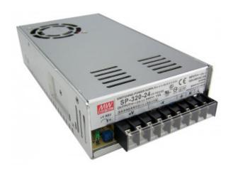
This is a power supply and wiring kit to power the Koolance <u>EXC-450</u> or <u>VLX-450</u> chillers from an AC outlet. DC and AC wires are included (AC plug is for North American outlets). The power supply is auto-switching, 100-240VAC 50/60Hz input to 24VDC output. It is rated to 312W, with PFC, and is CE and UL labeled. The size is approximately 9in x 4.5in x 2in (230mm x 115mm x 50mm).
