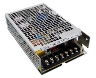
This is a power supply and wiring kit to power Koolance ALX cooling systems from an AC outlet. DC and AC wires are included (AC plug is for North American outlets). The power supply is auto-switching, 100-240VAC 50/60Hz input to 12VDC output. It is rated to 100W, and is CE and UL labeled. The size is approximately 6.25in x 4.75in x 1.5in (159mm x 121mm x 38mm).
