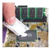
Once loosened, remove the original heat sink. Apply a thin layer of thermal interface compound onto the chipset if necessary.
