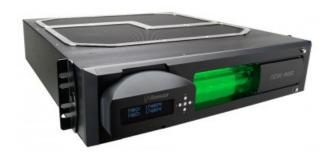
ERM-3K3UC is a rack-mountable or free standing ambient liquid cooling system. This model contains a large nine x 120mm fan copper/brass radiator, providing roughly 2400W of cooling with a 25°C ambient delta. Just add tubing, fittings, coolant, and connect to your cold plate(s).
