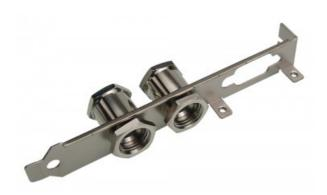
Dual panel-mounted socket threads for "internal/external" fittings on a computer chassis L-bracket. This also allows tubing sizes which are too large to fit through the chassis slot. Nickel-plated brass fittings with G 1/4 BSPP threads. This product may need to be temporarily disassembled during installation.
