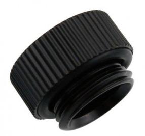
ADT-XMF-BK is a Male-Female G 1/4 BSPP (parallel) thread coupler. Among various applications, it could be used as a spacer for obtaining extra fitting clearance. The body height, not including the male threading, is 7mm (1/4in).
