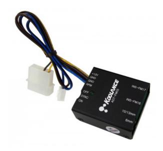
The Koolance Frequency Adapter multiplies <a href="INS-FM16">INS-FM16</a>, <a href="INS-FM16">INS-FM16</a>, or <a href="INS-FM19">INS-FM19</a> flow meter RPM signals to allow readability by most fan tachometer headers. A small green power LED on the unit blinks according to flow meter rotation rate.
