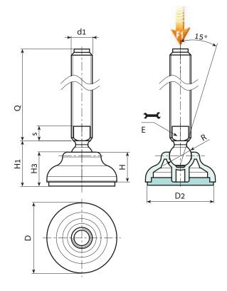
Version P910: Mounting foot with stem type B (with milled seat for wrench) and ball R15 - with SBS non-slip base
