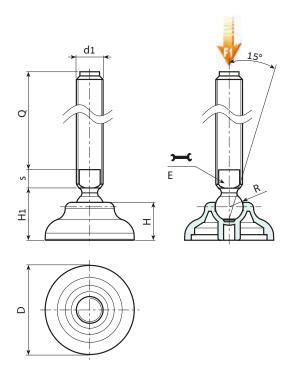
Version P907: Mounting foot with stem type B (with milled seat for wrench) and ball R15
