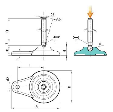
Version P708: Teardrop mounting foot with ground fixing - stem type B (with milled seat for wrench) and ball R
