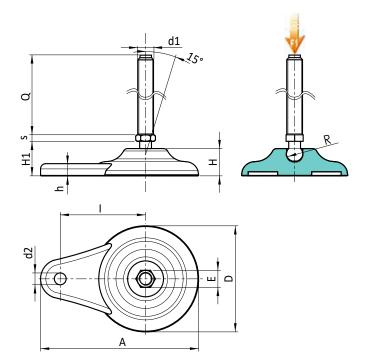
Version P700: Teardrop mounting foot with ground fixing - stem type A (with hexagonal base) and ball R12.5
